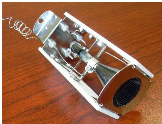
A continuous dynode particle multiplier detector.
